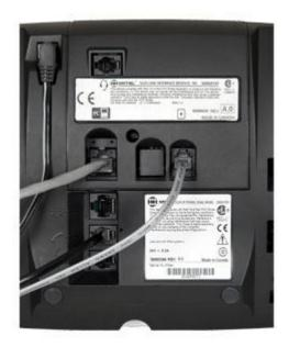
The Mitel Line Interface Module is a discrete optional module that integrates into the Mitel MiVoice 5324, 5330, 5340, or 5360 IP Phones and provides a separate connection to an analog line, like those found on DSL services.
